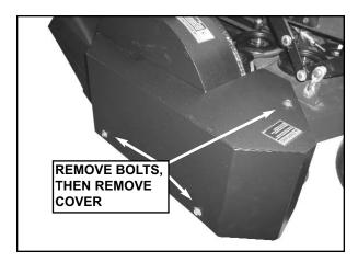
**STEP 6a:** Remove bolts securing impeller pulley cover to blower, and remove cover.
